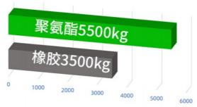
The green bar represents "Polyurethane (聚 )" with a load capacity of 5500 kg. The gray bar represents "Rubber (橡 )" with a load capacity of 3500 kg.
