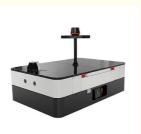
**Customized Table Size AGV Automated Guided Vehicle Incorporating Laser Navigation and Obstacle Detection Optimizing Logistics**
