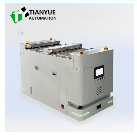
The Roller-type Transfer AGV is a state-of-the-art Smart AGV Robot designed to revolutionize material handling and transportation within various industrial environments. Engineered with precision and efficiency in mind, this advanced Automated Guided Vehicle offers unparalleled navigation accuracy of ±10mm, ensuring smooth and reliable movement throughout complex warehouse layouts and production floors.
