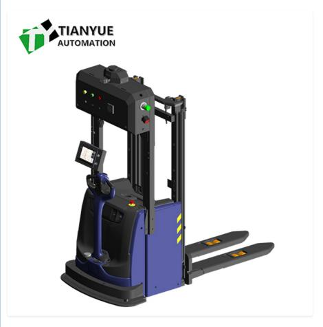
The Intelligent Unmanned Forklift represents a cutting-edge solution for modern material handling operations. Engineered with advanced automation technology, this heavy duty forklift truck delivers exceptional performance, efficiency, and safety for industrial applications. With a substantial load capacity of 1600KG, it's designed to handle demanding weights reliably, making it ideal for warehouses, manufacturing facilities, and distribution centers.
