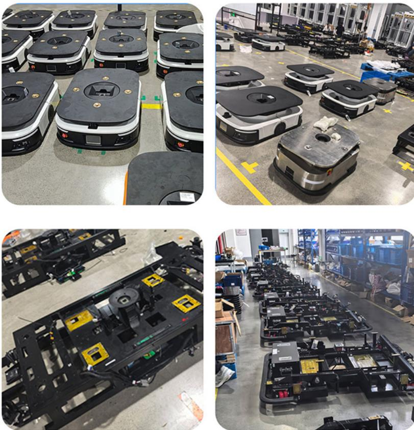
The TIANYUE Automated Guided Vehicle System is an advanced solution designed to revolutionize material handling across various industries. This AGV Robot is engineered with precision stopping capabilities of ±5-10mm and features an electromagnetic brake mode to ensure safe and reliable operation.
