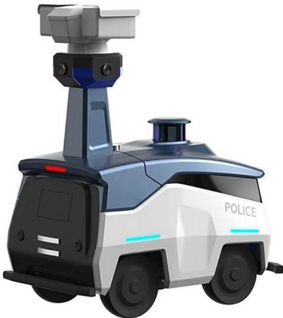
This advanced chassis delivers impressive performance with a maximum autonomous navigation speed of 1.6 meters per second, enabling efficient traversal across various terrains. The integrated intelligent detection system provides real-time obstacle sensing and environmental response, significantly enhancing vehicle safety and autonomy for complex outdoor navigation scenarios.
